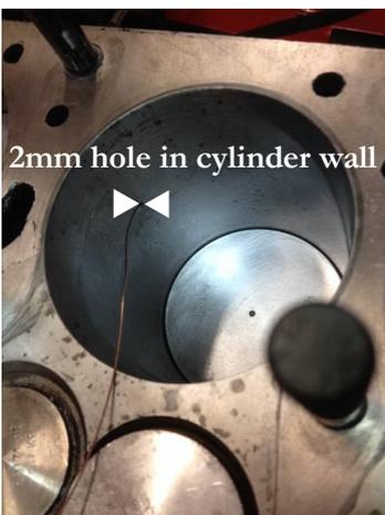
2mm hole in cylinder wall
