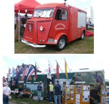
One particularly interesting vehicle was a 1967 Citroen model type H. Conceived as a delivery van, the H-van employed the characteristic Citroen front wheel drive to provide a very low loading height together with full standing. The distinctive corrugated panel work provided rigidity and permitted the use of thin-gauge steel sheet. Imported from France in August 2013 it is now a retired fire truck.
