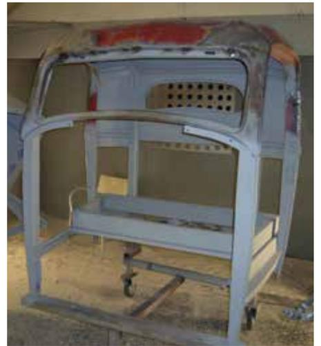
set about cutting out the required shapes. It was hard going and tiring work. It took about 5 hours over two days to cut the first piece, then taking several hours longer to cut the second piece, as the blade was blunt and kept ripping out of the machine. I also cut out a curved piece where the fuel tank filler pipe passed through.
